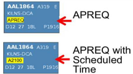
Fig. 13. Flight strip on RTC. (top: APREQ restriction without a scheduled release time; bottom: scheduled APREQ release time)
